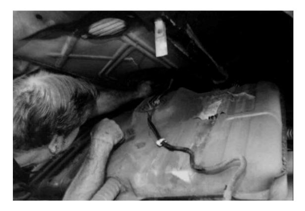
Before cutting the floor, the electrical connections to the fuel tank must be disconnected. Two fuel lines are cut and a third is unbolted prior to removing the tank. The straps that hold the gas tank can either be unbolted or cut with an air chisel. We will reposition the tank later.
