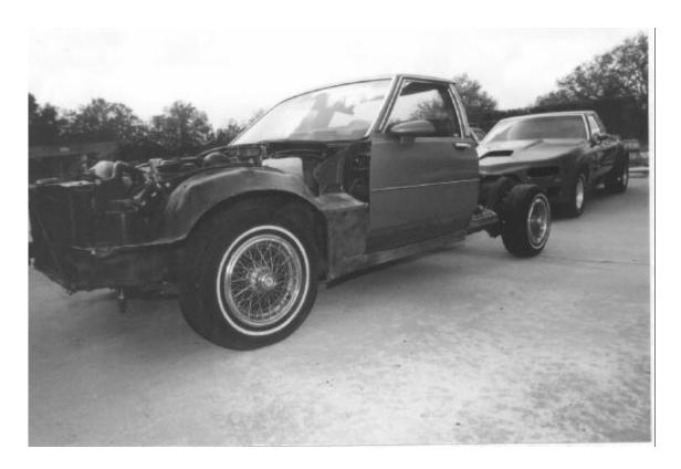
Here's a before and after shot to motivate you! Don and John lift the new fiberglass rear clip into place. To establish the correct support for the bed, 2X4 wood spacer blocks, about 10" high, are positioned temporarily on the frame rails. The height of these blocks is slightly variable and the exact size is determined by how well the front edge of the rear clip matches the rear edge of the door.
