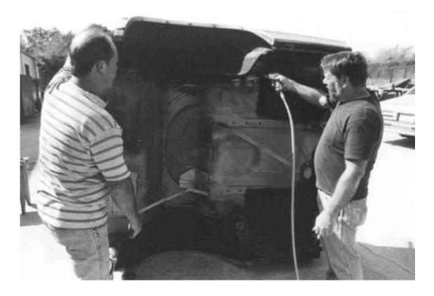
Before the rear of the car is disposed of; Don uses the air chisel to free the two, square threaded washers that will later be used for the body mounting bolts. A grinder or a Sawzall could accomplish the same thing.
