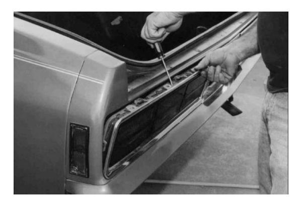
The taillight panel has plastic nuts in the trunk that have to be removed. After labeling the bulbs, the rear wiring harness that supplies electricity to all the rear lights is detached from the main harness. The main wiring harness is pulled back through the rear seat opening and secured out of the way when the floor is cut. Plastic ties will secure the wiring harness to the driver's side chassis rail once the rails are cut. The Caprice taillights are removed and saved for reuse later.
