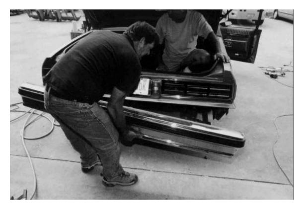
The rear bumper is removed using the same technique as the front bumper. The fold down license plate is detached and saved for later use. It will be reinstalled on the new rear clip.
