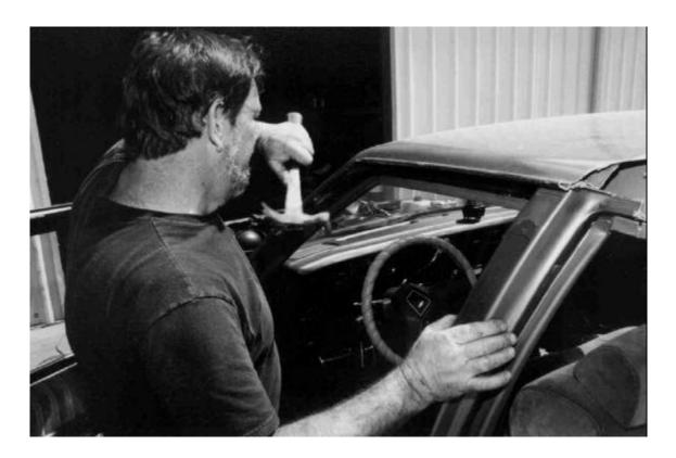
After removing the Caprice's chrome trim from the drip molding, Don uses a hammer to flatten the rain gutter against the roof. Once it is flat, it will be filled with Bondo and molded into place. Here's an advanced look at what the roof will look like when it is blended to the fiberglass clip.
