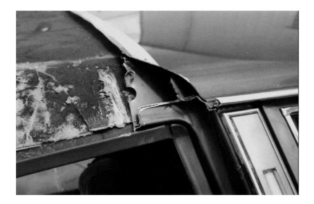
Before the rear clip is lifted into place, a second roof cut is made, trimming the edges around the door pillar on a 45 degree angle. The edges are ground smooth to ensure the fiberglass clip will slide easily into place.
