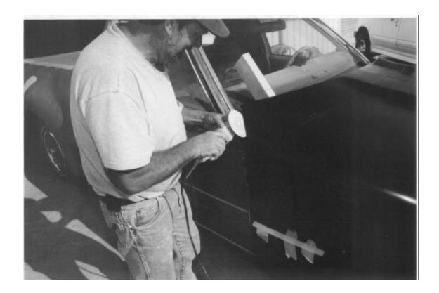
Remember that fiberglass is as easy to grind down as it is to build up. It's easy to shape and not at all like metal. There are several trim-able edges intentionally designed into the kit. The area on the rear clip that mates to the rear edge of the door must be carefully shaped for a perfect fit. The rear portion of the front clip is also adjusted to fit the front edge of the doors. Some use a paint stick wrapped in 200 grit paper to get accurate cut lines.
