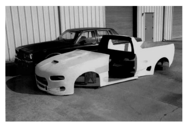
The four-piece kit is simplicity itself. Up front there is a tilt forward front clip, the rear is a one piece pickup bed, and a pair of rocker panels join the two. The Chevrolet Caprice donor car used for this project is an '89 but Caprice, Bonneville, and 01ds88 in the years from 1980 to 1990 are readily available and inexpensive.
