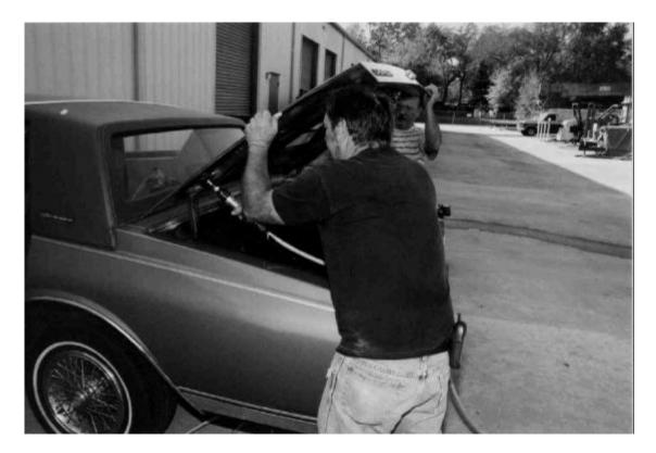
The trunk is unbolted to lighten the load when the rear clip is removed. A strip of masking tape, roughly following the contours of the rear floor pan, is laid in place as a guide for the cut. By following these lines, the body mounting bolts located roughly in the center of the rear door, will remain to ensure that the cab stays rigidly mounted to the chassis.
