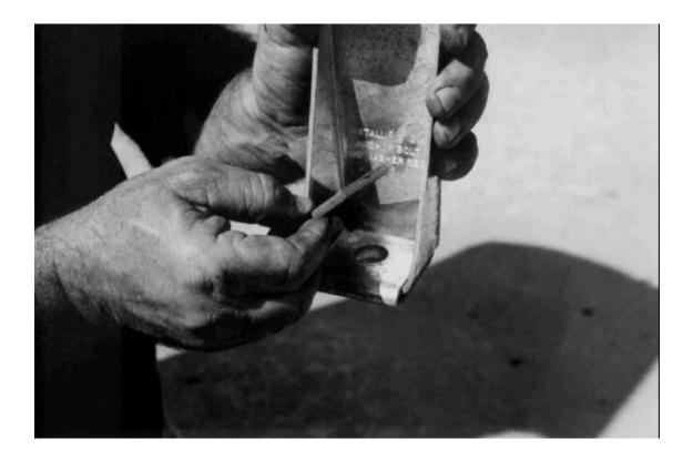
The HTT- 16 Simpson Strong Tie connecter brackets are actually commercial construction items used in home building. The square threaded washers, previously removed from the underside of the body, fit perfectly inside. Two Simpson connecters are bolted to the rear of the chassis, in the original holes and using the original body mounting bolts. The bed will later be fiberglassed to the connecter brackets.
