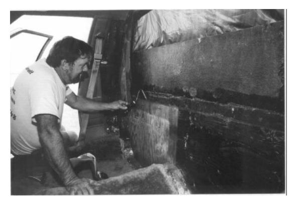
The new interior wall has to be glassed in (We used plywood cut to fit.) to close off the rear. This kit has a design change that moved the rear wall of the kit back about 5" compared to the prototype for additional leg room and space for a competition stereo. There is also a storage box built in under the pickup bed floor.
