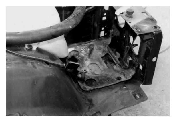
The battery must be relocated to accommodate the tilt forward front end. The tray is removed and will be relocated either on the rear chassis member under the pickup bed or the front fender on the driver's side. The headlight brackets must be trimmed to allow clearance for the tilt-forward hood. An air chisel or Sawzall makes short work of the process but a hacksaw can get the job done.
