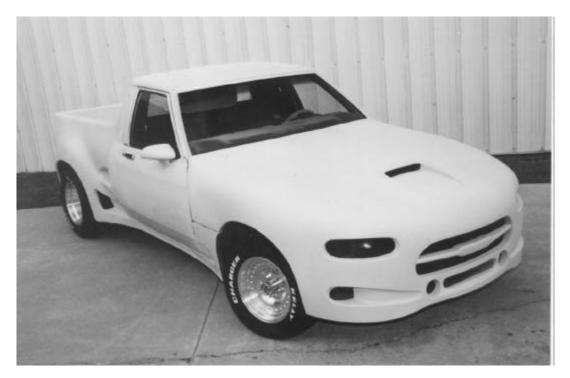
These are the final shots, showing the kit in primer on a set of 15" Centerline wheels. We accomplished the basic body mounting procedures in two six hour days. Starting on Saturday, the front and rear clips were temporarily in place by 2 PM Sunday afternoon. While there was plenty more to do, the basics were in place. The weight savings over the stock Caprice (3820 pounds) was a substantial 700 pounds. The reduction made the stock 305 V-8perform like a big honkin' 350!
