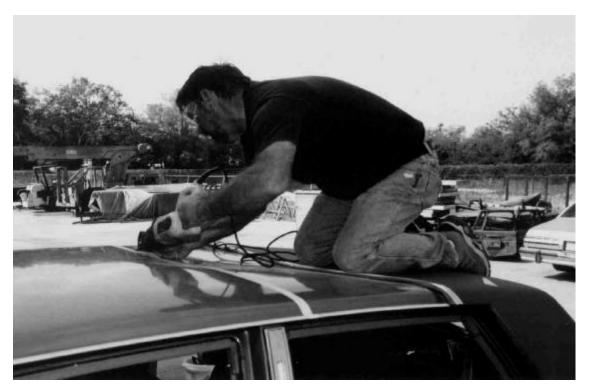
Since the Caprice had a new head liner, we decided to save it. Using a box cutter knife~ we cut the head liner about 14" to the rear of the interior light. Next, we added a taped mark on the roof that went from side to side, just behind the front door pillars. We will keep the front doors and the pillars that support the rear doors, cutting the roof just behind the pillars. As Don cut the roof from above, John held the head liner back, being careful to avoid the saw blade.
