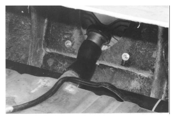
The fold down Caprice licence plate holder is reused. Simply screw it into place in the recessed opening on the rear clip. The stock factory goose neck on the gas filler is trimmed to fit and the original gas cap reinstalled.
