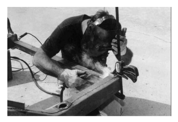
A section of 2" rectangular steel tubing, about 4" long, is cut to fit the distance between the frame rails Weld it into place making sure that it is aligned with the lower portion of the frame rails to allow clearance for the gas tank filler to pass over the top. Later we will add triangular gussets to further reinforce the frame. The gas tank is repositioned between the frame rails and rests on a  $1.5" \times 1.5"$  angle iron shelf.
