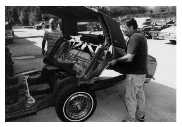
Before the rear half of the body can be lifted off the chassis, the exhaust heat shield from the muffler must he cut away. It's tack welded into place and either the Sawzall from above or the air chisel from below can eliminate the connection. Here's what the Caprice chassis looks like, stripped for action.
