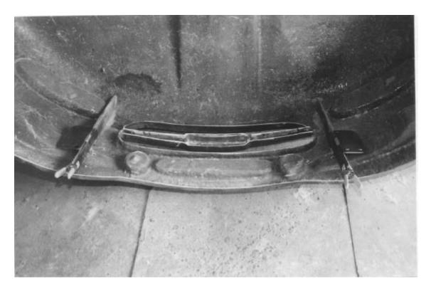
The tilt front end comes with steel mounting supports built-in. The clip is lifted in place and supported temporarily with a short length of 2X4 laid across the radiator. The rear of the clip is aligned with the front edge of the door and the top edge of the rocker panel. If there's a gap at the bottom of the doors, the 2X4 support needs to be trimmed. If the gap is at the top add shims until the clip matches the door edge evenly.
